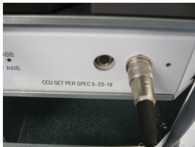
10. Connect the camera cable to the receptacle next to the focus cable on the instrument control module. The connector on the camera cable is indexed to its receptacle by a slot at the bottom of the connector. Make sure the slot aligns properly with the receptacle and carefully thread the connector into the receptacle until it is tight.
