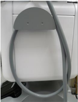
5. Gently unsnap and remove the front cover from the system by prying along the cover edges and drawer opening using only fingertip pressure.
