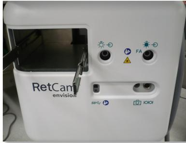
6. Before connecting the handpiece harness, ensure that the main power switch on the back of the cart is off.
