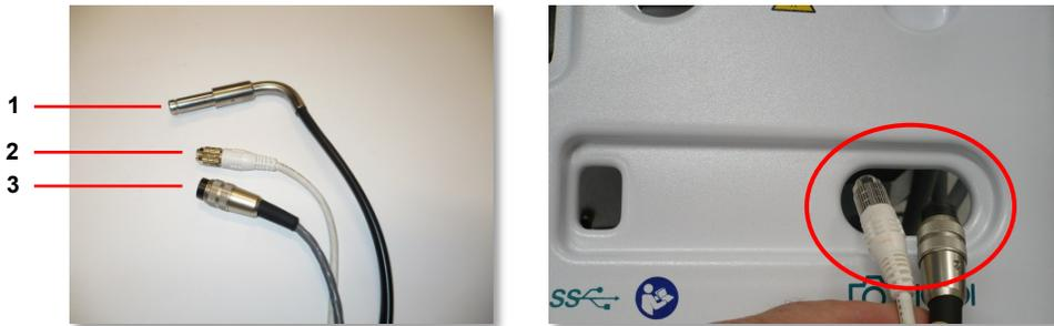
8. Connect the handpiece camera and focus cables to their corresponding ports in the instrument control module behind the front cover.
